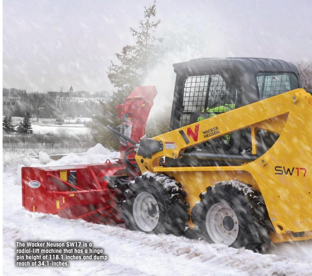
**The Wacker Neuson SW17 is a radial-lift machine that has a hinge pin height of 118.1 inches and dump reach of 34.1-inches.**
