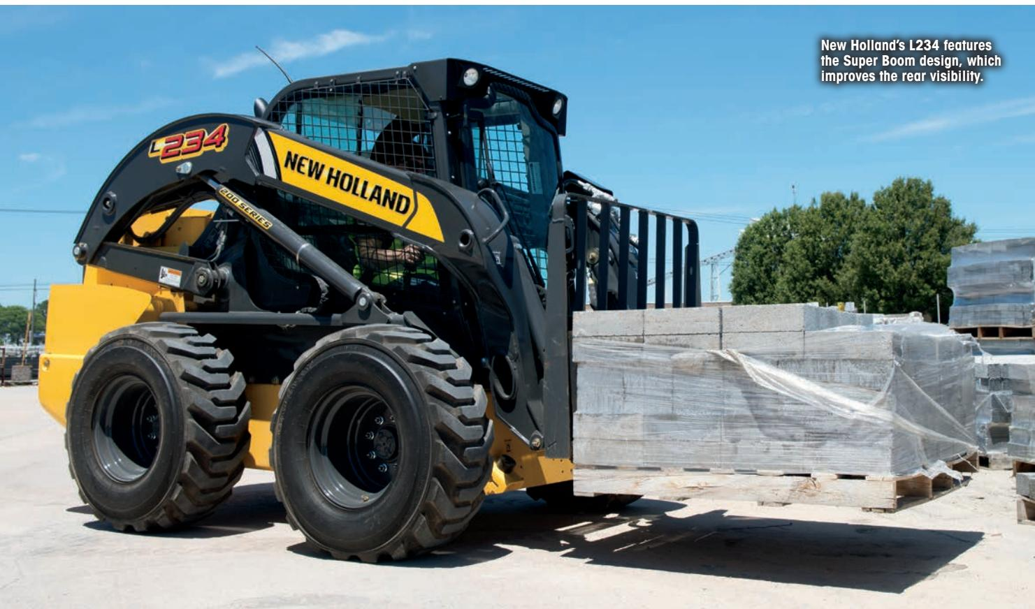
New Holland's L234 features the Super Boom design, which improves the rear visibility.
